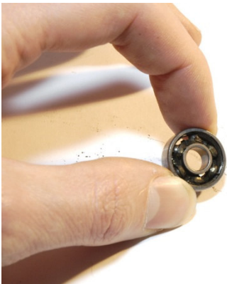
On a standard double rubber sealed bearing, the same thing happened: used balls and mix of oil and dust. The bearing couldn't work anymore.
