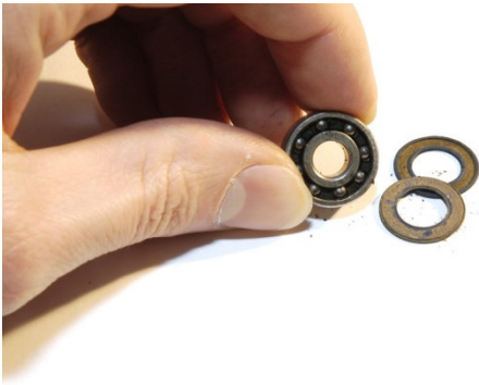
Balls are very used and dust mixed with oil formed a kind of paste.
